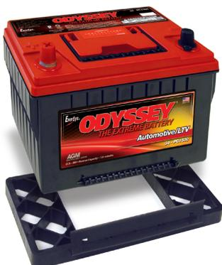
Optional height adapter may be used on 34-PC1500 models for installations where a group 24 or group 27 is required. Snap the adapter securely into place on the bottom of the 34-PC1500 battery. In some installations, the 34-PC1500 model with this adapter may be used to replace a group 24F or 27F depending on required cable length.
